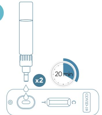
Put two drops into the sample well of the test cassette, and start the timer.
